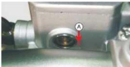
1. With the motorcycle in the upright position, check the brake fluid level. It should be above the indicator mark (A) on the master cylinder. If the level is below the mark, check the brake pads for wear. Worn out pads should be replaced. If the brake pads are not worn out, check your brake system for leaks.
