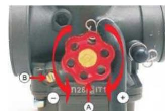
The idle setting of the carburetor has a big influence on the vehicle's starting behavior, on stable idling and on the vehicles response when the throttle is opened. An engine with a correctly set idle speed is easier to start than an engine with the idle speed set incorrectly. The idle speed is adjusted with the idle speed adjusting screw.
