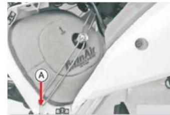
1. Detach air filter holder **Q** at bottom and move it to one side.
