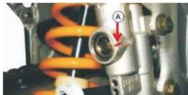
1. With the motorcycle in the upright position, check the brake fluid level. It should be above the indicator mark on the master cylinder. If the level is below the mark, check the brake pads for wear. Worn out pads should be replaced. If the brake pads are not worn out, check your brake system for leaks.
